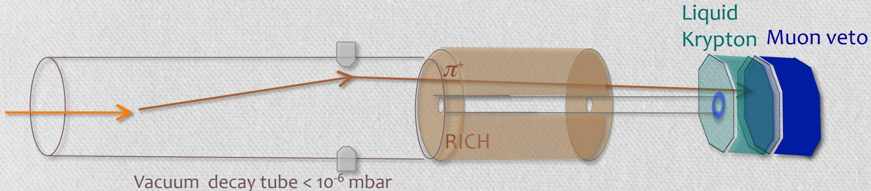
For 1-track sample, need to precisely identify the track as a pion
