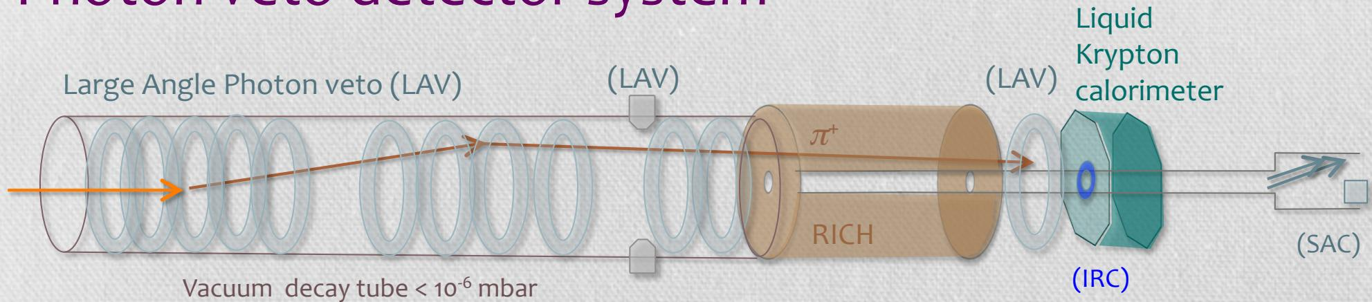
4 different types of detectors: LAV, LKr calorimeter, Intermediate ring calorimeter (IRC) and small angle calorimeter (SAC)
