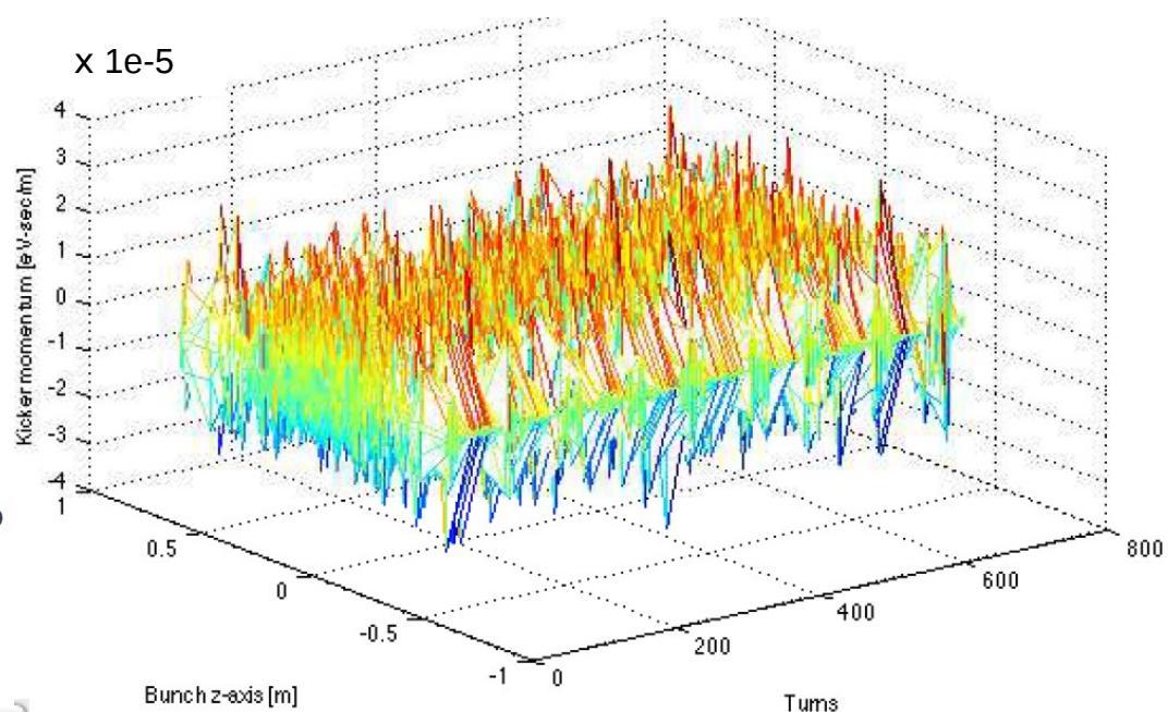
Same scale: Low feedback power is required to stabilize the beam in the presence of electron cloud
