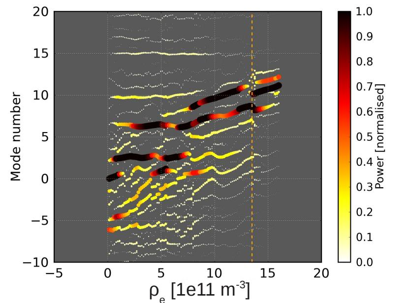
$$500\text{MHz} - \rho_e \approx 6\text{e}11 \text{ m}^{-3} - \text{gain} = 6\text{e}-3$$
