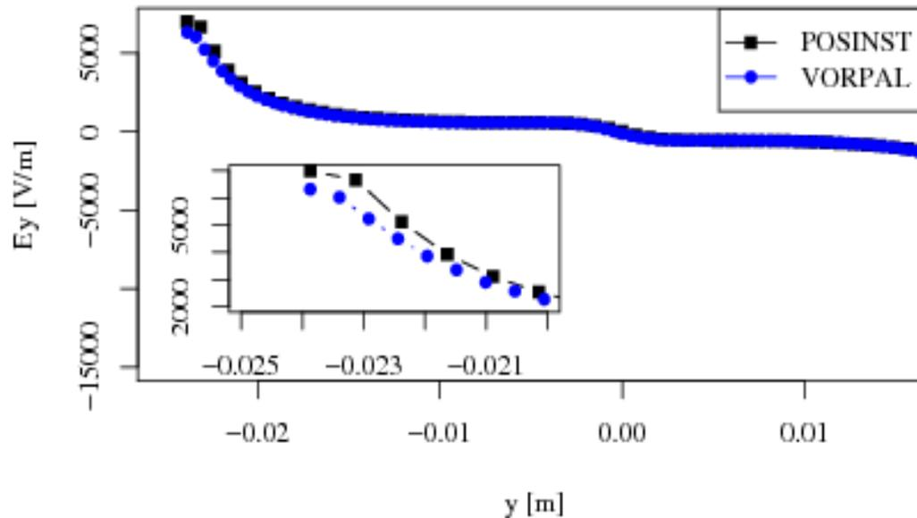
Electric field, vertical component, as a function of the vertical from the center of the beam pipe.
