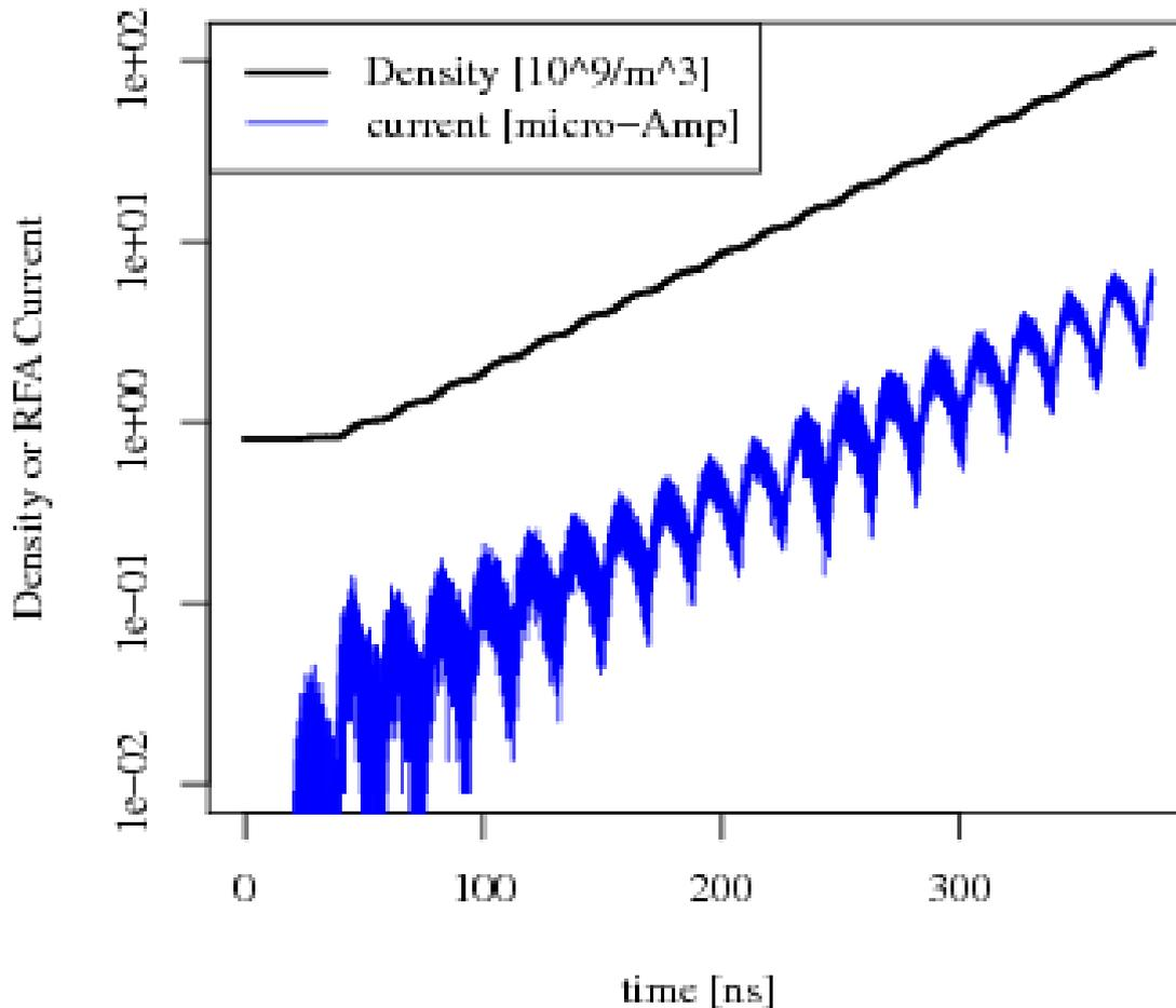
Implementation in VORPAL, for the nearly  $\phi$ -symmetric case: Count the number of macro-electron hitting the wall, rescale by the ratio of the geometrical aperture of the RFA to the beam pipe surface.
