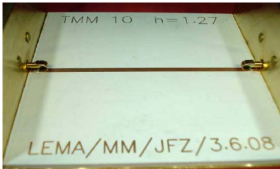
TNC coaxial to microstrip transition (LEMA/EPFL)
