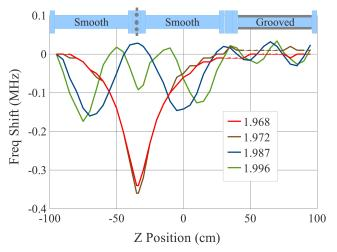
In a measurement with two smooth sections of beam-pipe at the drive point, a cutoff mode response is observed. This is due to the design of the BPM.
