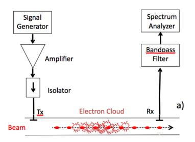
The original idea was to propagate microwaves through the beam-pipe as if it were a waveguide.
