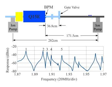
At 15E in CESRTA, the lowest resonance is much lower than might be expected of a rectangular cavity.
