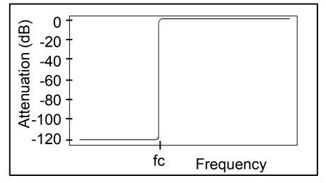
In an ideal waveguide, microwaves do not propagate at frequencies below the cutoff frequency.
