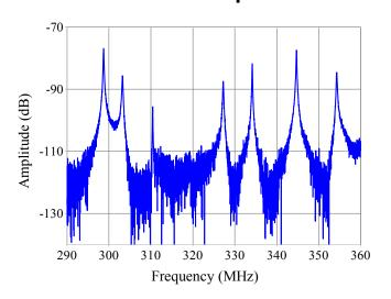
The positron ring at DA $\Phi$ NE shows strong resonances, but the spacing of the peaks needs careful analysis.
