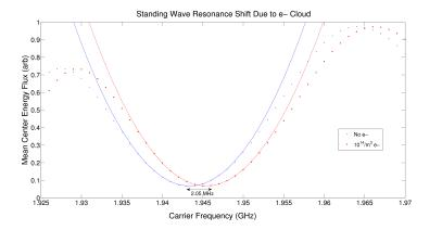
The shift in resonant frequency for A density of 10<sup>14</sup> m<sup>-3</sup>, is about 2 MHz. This also agrees with Equation 1.
