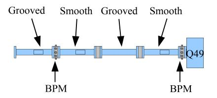
In the L3 chicane region, there are sections of both smooth and grooved round beam-pipe
