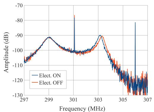
The amount of frequency shift varied from peak to peak. Here the lowest frequency resonance is unshifted, while the next peak is shifted by 200kHz as the clearing electrodes are turned OFF/ON.
