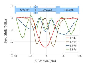
With smooth and grooved beam-pipe at the drive point, the first two resonances are mostly within the grooved section. the cutoff frequency of the grooved pipe is lower than that of the smooth pipe which explains the effect.
