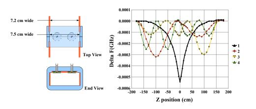
But if the drive flange is modified, the lowest resonance has a very different characteristic. The field decreases exponentially with distance from the drive point (cutoff mode).
