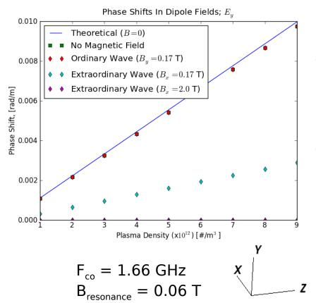
With larger dipole fields, such that the cyclotron frequency is much higher than the TE wave excitation, there is a reduction in the phase shift of the x-wave.
