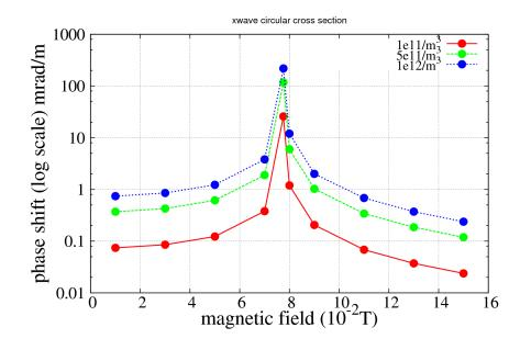
When E of the TE wave is perpendicular to the dipole field (x-wave) there is a magnification of the phase shift. This is due to the proximity of the cyclotron resonance. The TE wave frequency was 2.17 GHz
