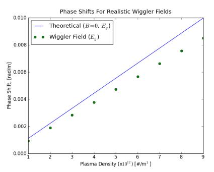
The simulated phase shift through a wiggler gives a somewhat reduced phase shift even Though E is parallel to the main wiggler field.
