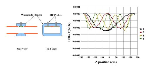
With a drive flange that matches The inner dimensions of the waveguide, the frequency shift vs. position shows the expected sequence of half wavelengths.
