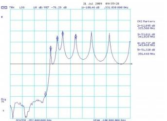
At the APS (Argonne National Laboratory), resonances are produced between bellow end flanges of the vacuum chambers (plot courtesy of Robert Lill). This response also matches that of a rectangular cavity.
