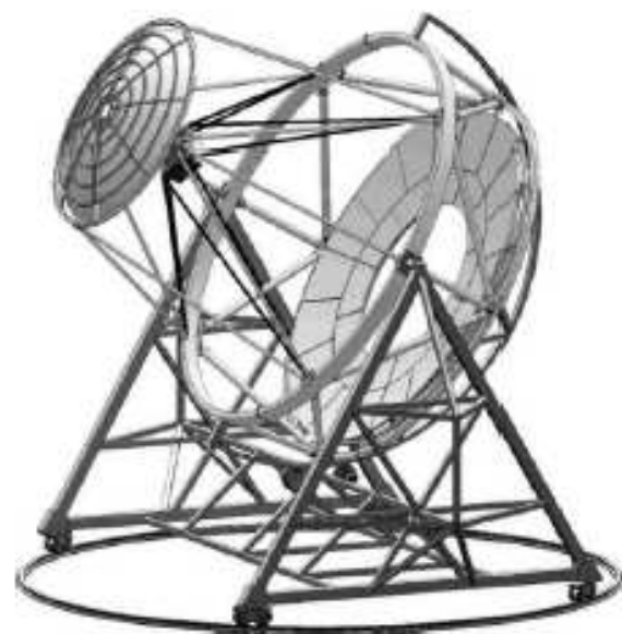
Fig. 5. – Top left: concept of a 23 m diameter LST with parabolic dish and f/d=1.2 . Top right: concept of a 12 m diameter MST with a Davies-Cotton dish and f/d=1.4 . Bottom left: concept of a 6 m diameter SST with a Davies-Cotton dish and f/d=1.4 . Bottom right: concept of a dual mirror Schwarzschild-Couder telescope.
