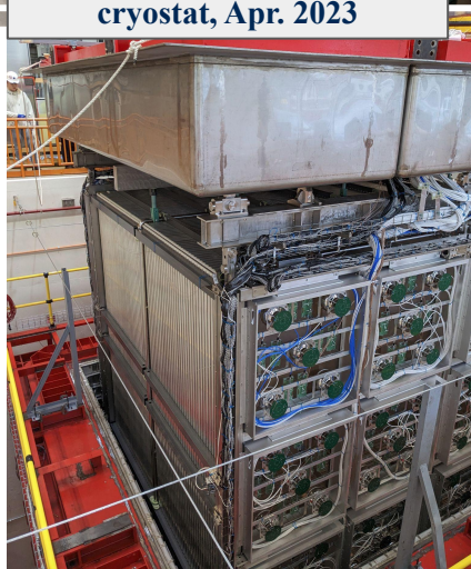
Detector inserted in the cryostat, Apr. 2023
