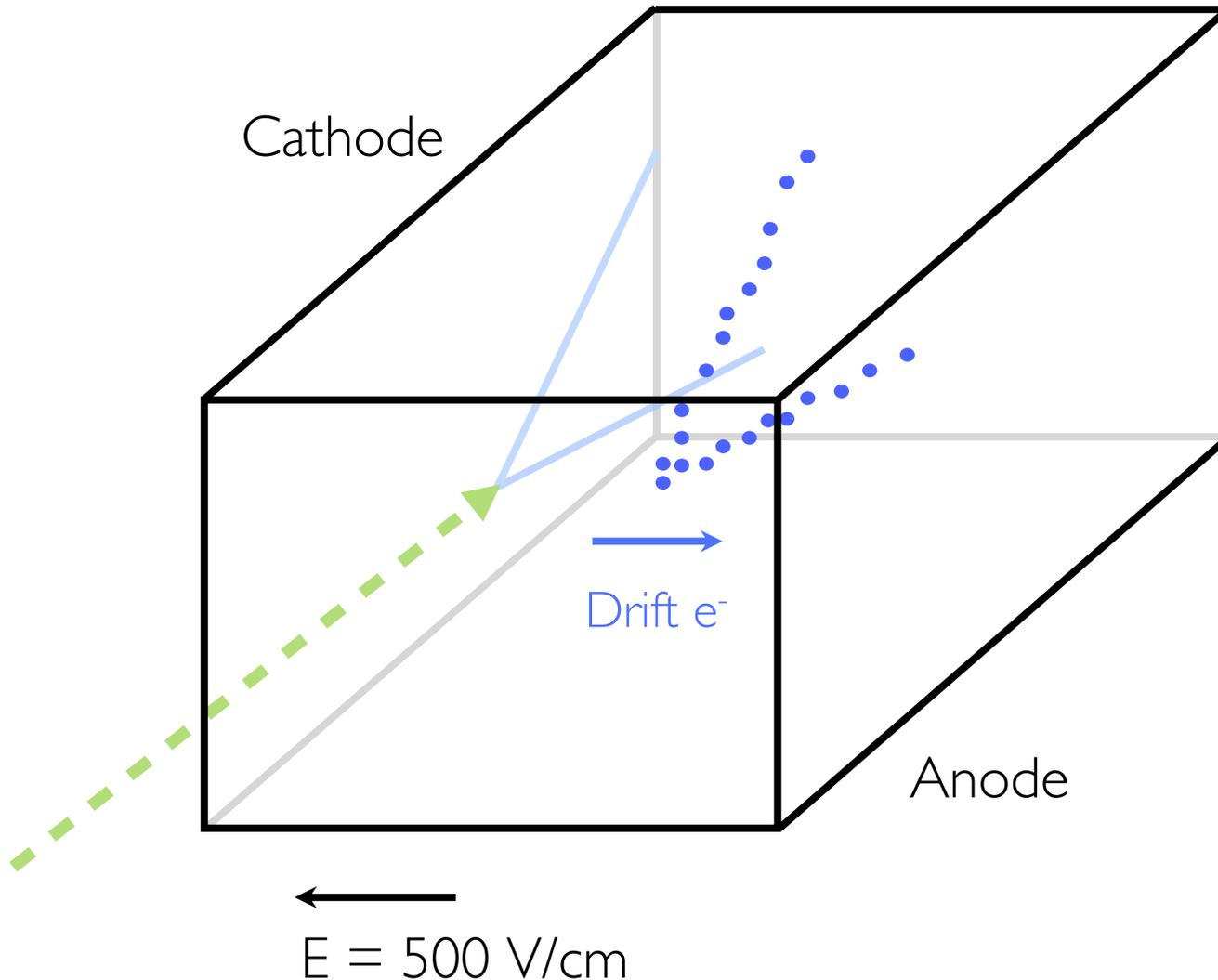
The ionization electrons produced by each ionizing particle are transported by the uniform electric field and can be detected in the anodic plane placed at the end of the drift path (maximum drift time 1 ms)
