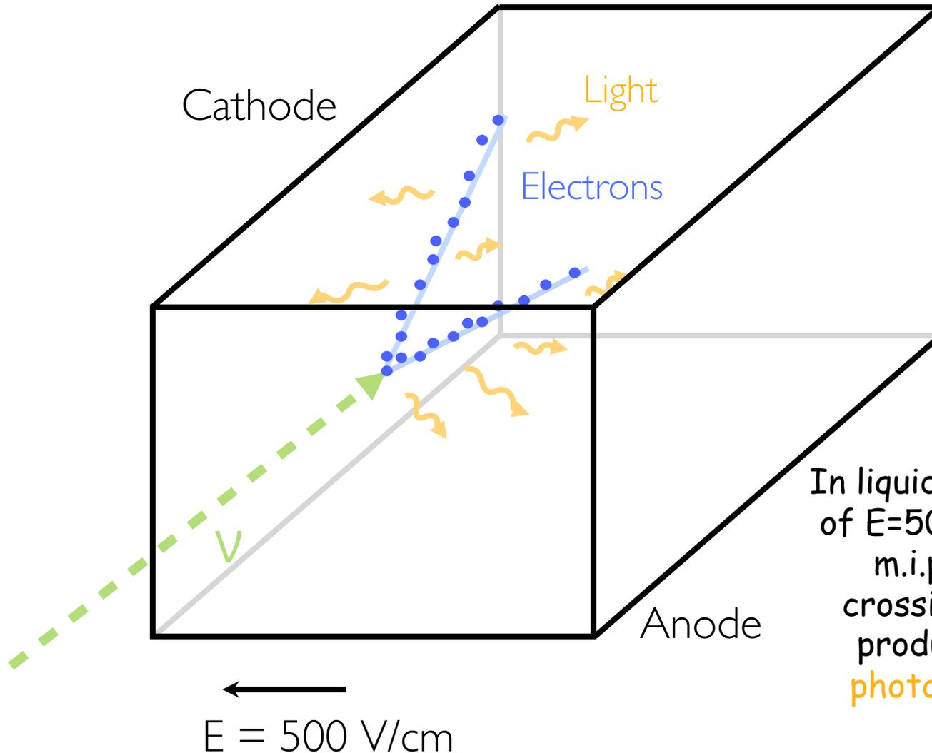
In liquid Argon, if an electric field of  $E=500 \text{ V/cm}$  is applied, a muon m.i.p. ( $dE/dx \sim 2 \text{ MeV/cm}$ ) crossing 1 mm of the detector produces  **$\sim 4000$  scintillation photons** and  **$\sim 5000$  ionization electrons**
