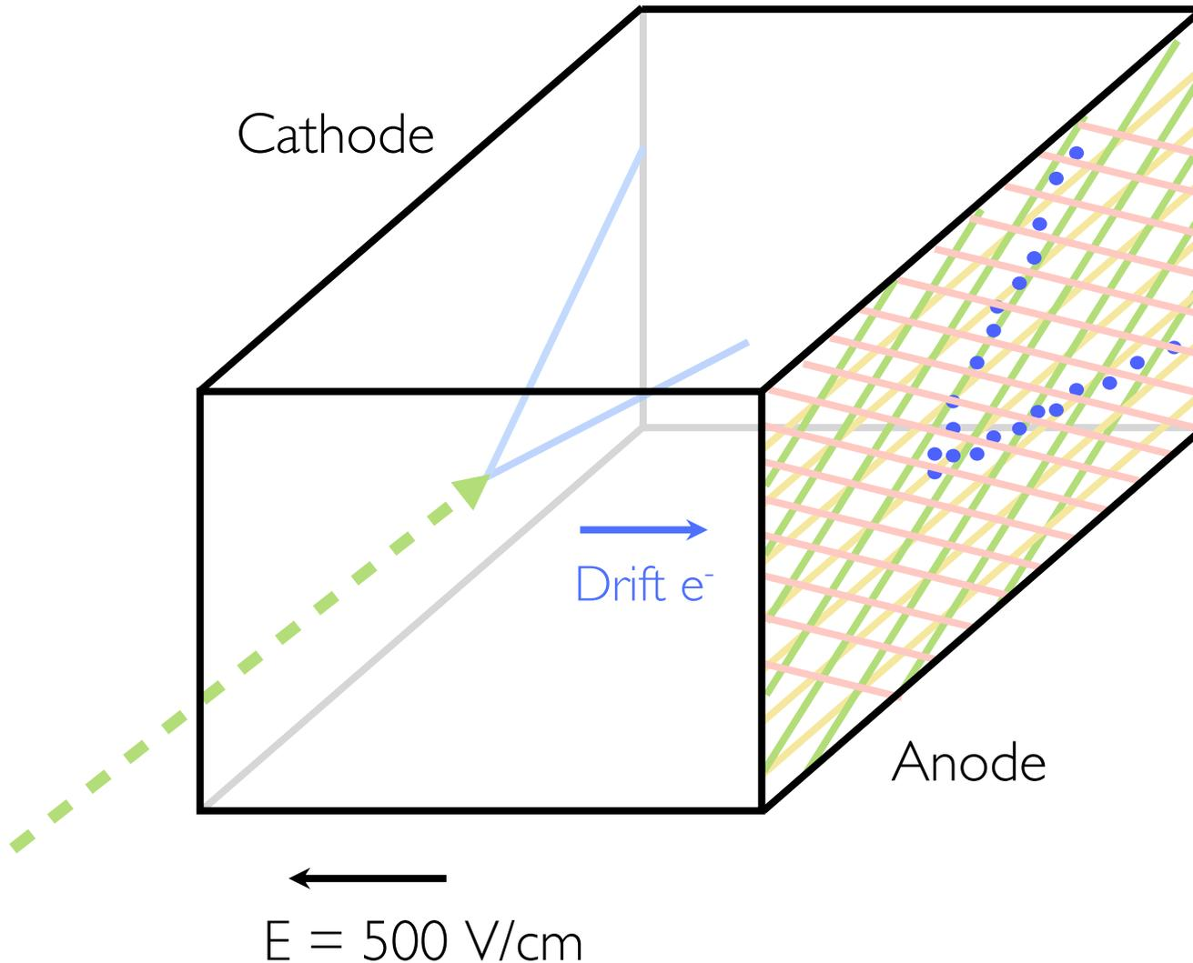
The ionization electrons are then detected by the 3 anodic wire planes providing simultaneous different projections of the same event. The information from these three projections allow a precise reconstruction of the recorded particle trajectories and a precise calorimetric measurement.
