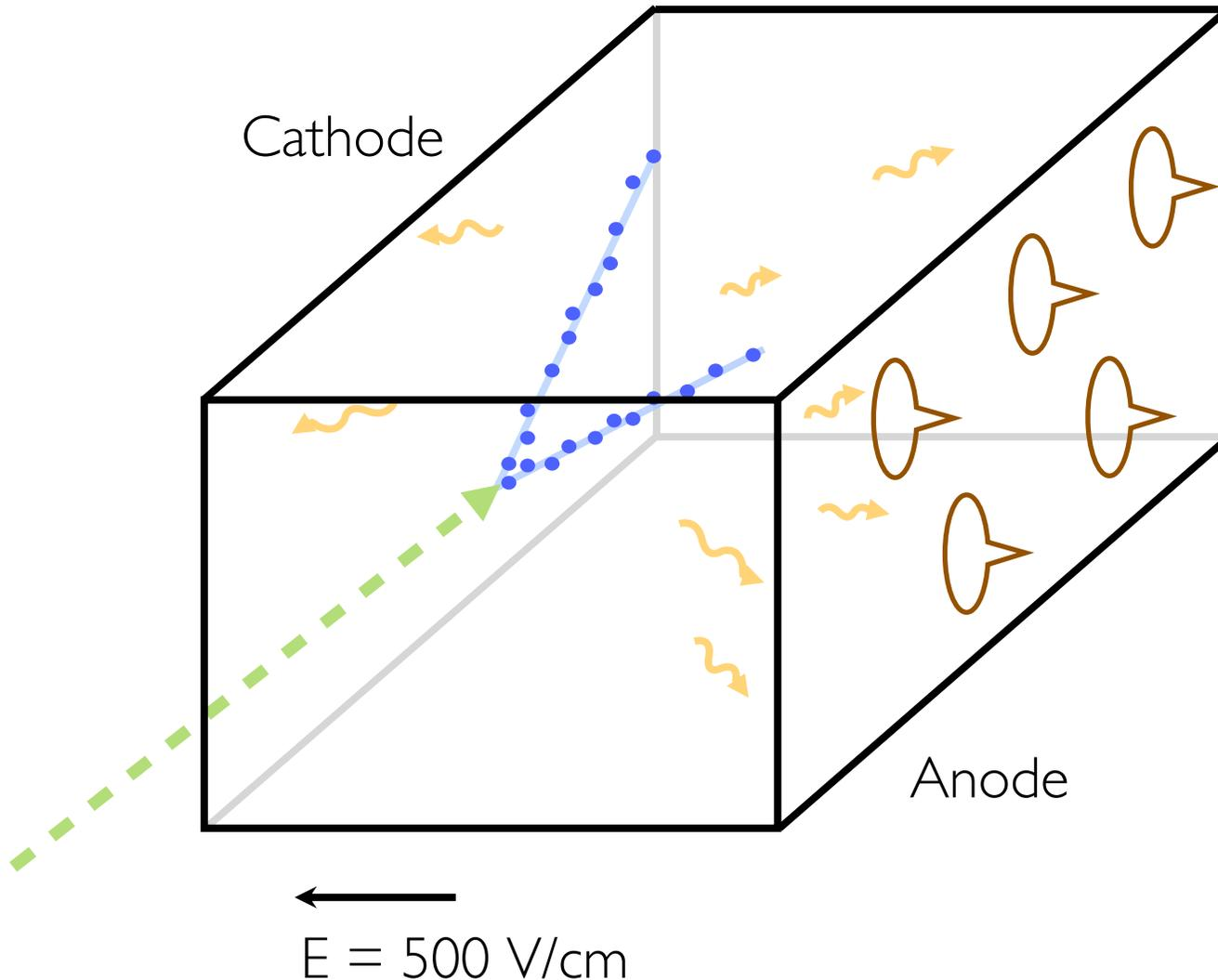
Since the liquid Argon is transparent to its own scintillation light, this light propagate inside the detector and can be collected by PMTs: this signal is the basis to recognize that there has been a particle interaction in the detector (**TRIGGER**)
