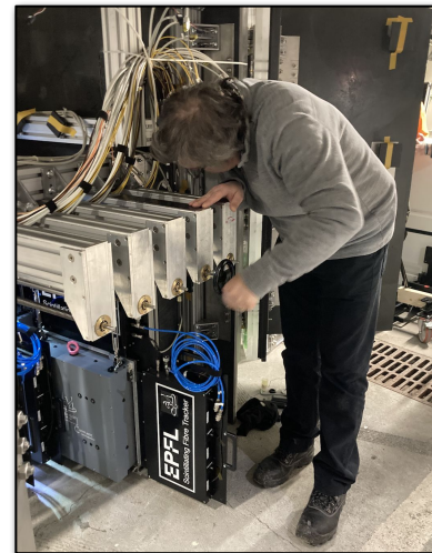
Emulsion target installation
