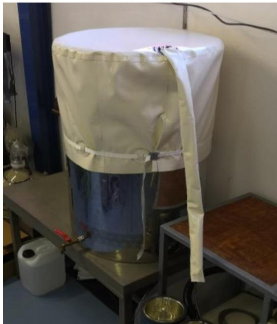
A small tank (300 l) is filled with pure water and a 5'' PMT is inserted in the bottom of it. Spectra taken with a PMT alone as well as in coincidence with two scintillators plates in different configurations.
