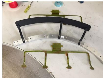
Handling frame arcs metrology with Gantry and confocal chromatic confocal optical pen
