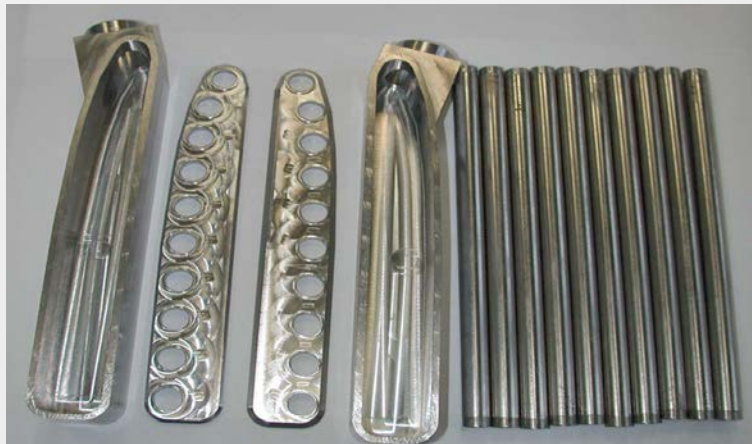
2. Zr cooling system manifold & collector plates
