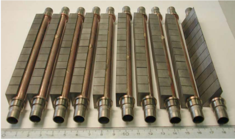
1. Be-tile brazed cooling pipes with Zr adapters
