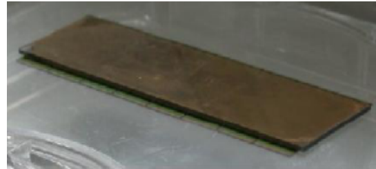
2cm x 6.3cm diamond sensor TiW metalization by IZM
