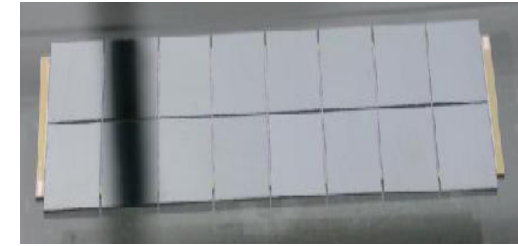
16 FE chip FE-I3 SnPb bump-bonded to diamond sensor by IZM
