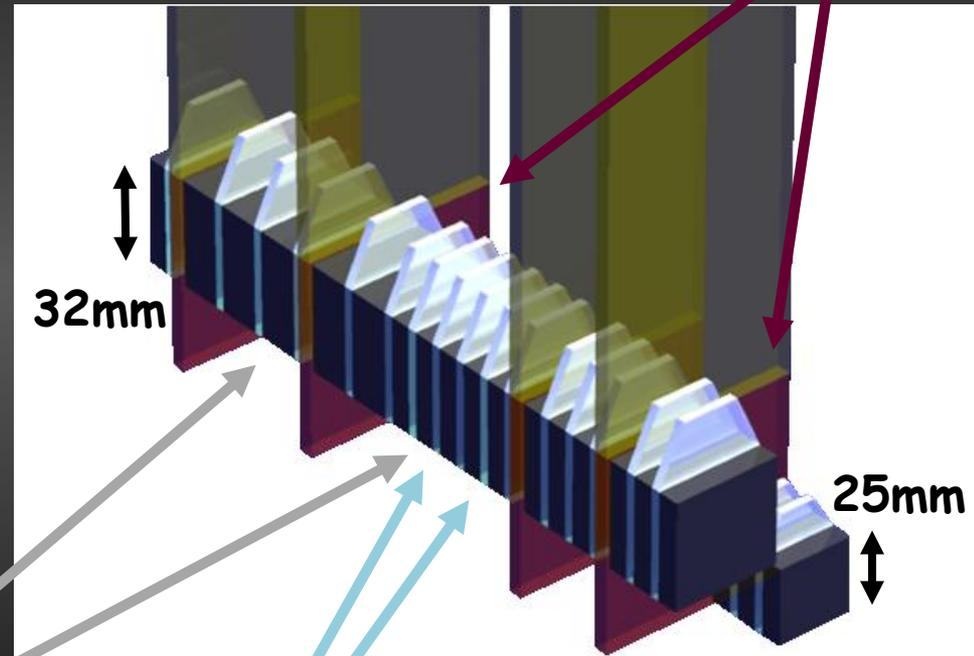
**Plastic Scintillator:** 16 layers, 3 mm thick, trigger and energy profile measurement
