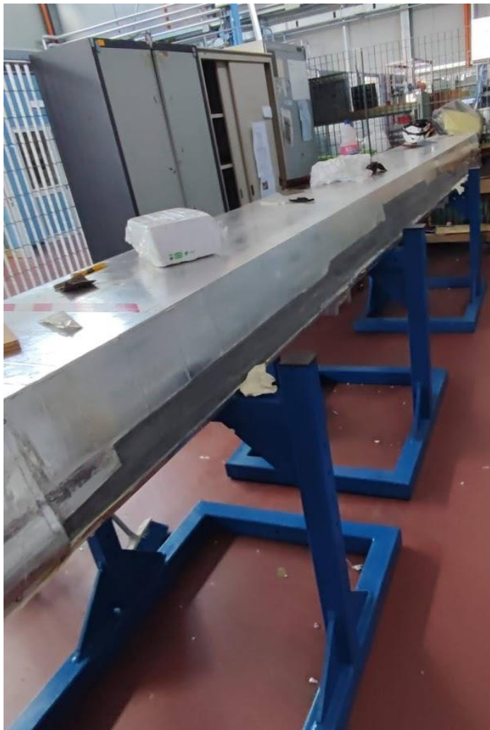
New wrapping with Aluminum/Glass Cloth tape
