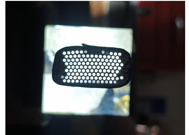
Gluing of 6 delaminated modules after test of adhesives on Lead-fibres mock-up
