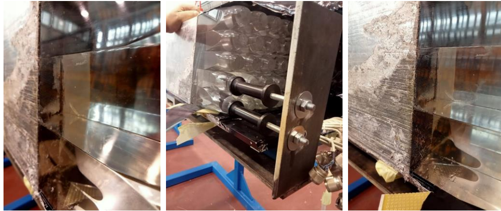
Gluing of 2 light-guides in 1 module
