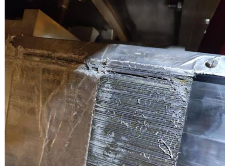
Gluing of 6 delaminated modules after test of adhesives on Lead-fibres mock-up
