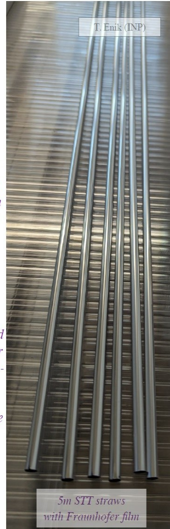
Production of 5m straws with Fraunhofer film and ultrasonic welding
