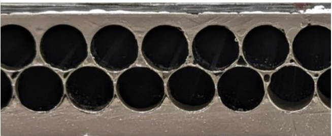
4. Conductive paint covering
