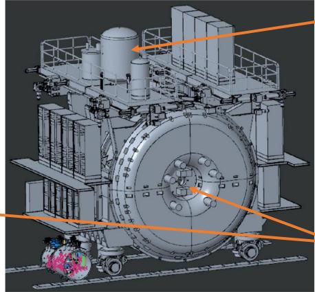
Proximity cryogenics of GRAIN (preliminary Layout)
