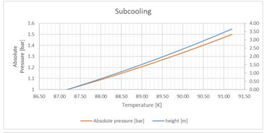
In the table above and in graphs on the right it is shown the obtainable temperature margin by means of the hydrostatic height of the LAr. The subcooling is necessary in order to reduce/avoid the production of Ar bubbles coming from the electronics immersed in LAr.
