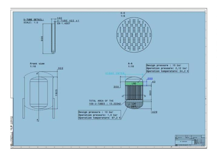
This U-tube heat exchanger is dimensioned for 1500 W.
