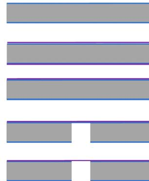
1. 280  $\mu$ m thick wafer with Silicon Oxide
