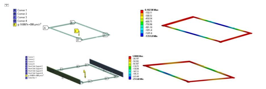
In the horizontal setup the vertical deformation could be reduced from 1.35 mm to 0.25 mm
