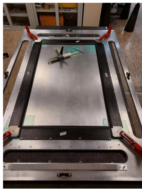
Gluing a Supporting frame
