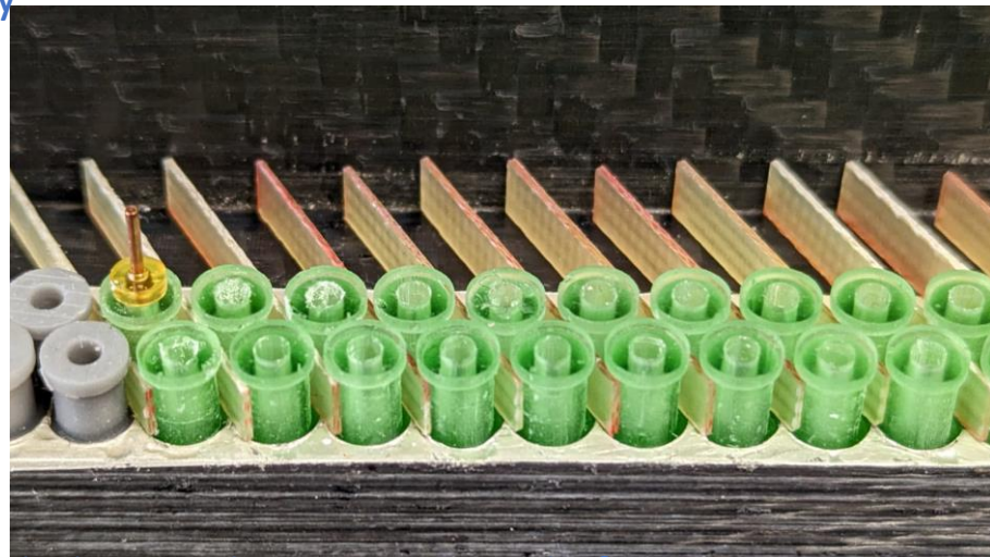
End plug are kept temporarily for wire insertion.
