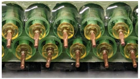
Final sealing with stycast glue poured around the neck of the end-plugs with the module in vertical position.
