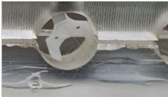
MA tooling developed for COMPASS to glue spacers on 4m long wires before insertion into straws
