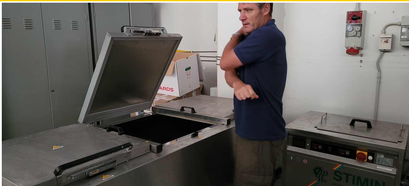
Large ultrasonic washing machine available at LNF to wash and clean PMTs and/or bases
