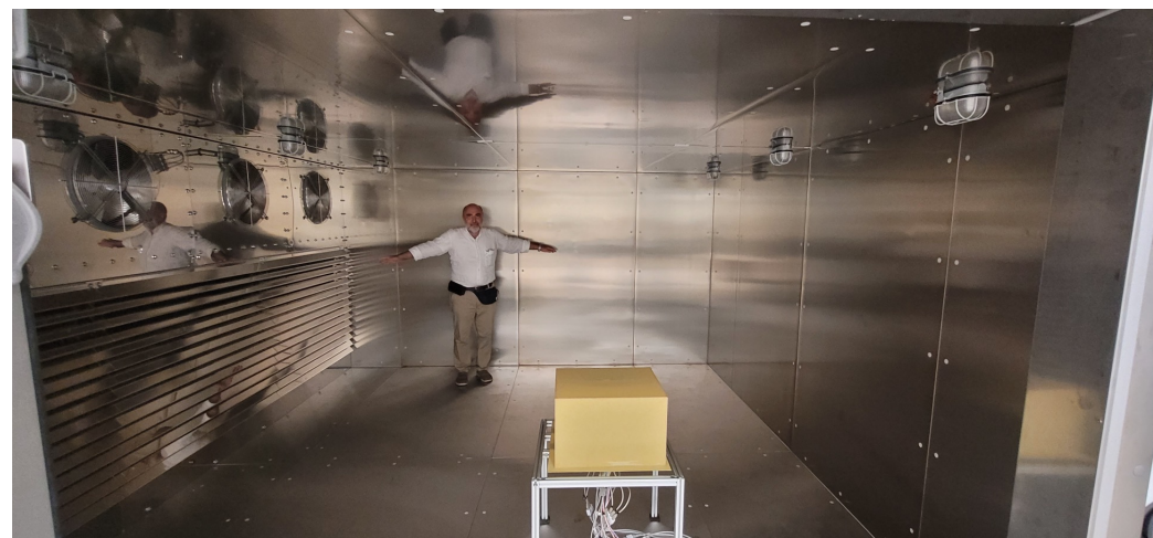
Large climatic room available at LNF to dry PMTs and/or bases
