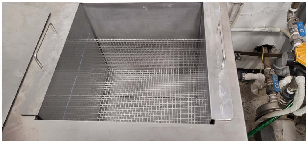
Large ultrasonic washing machine available at LNF to wash and clean PMTs and/or bases
