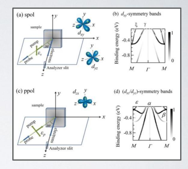
Using polarization to selectively excite orbitals in  $EuFe_2As_2$  pnictide
