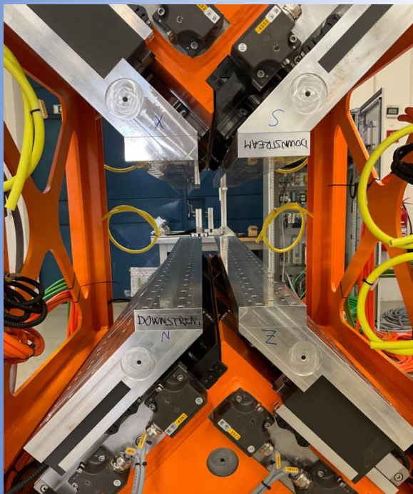
APPLE X undulator allow for polarization tuning (from linear to circular)
