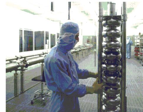
Cleanroom handling of niobium cavities
