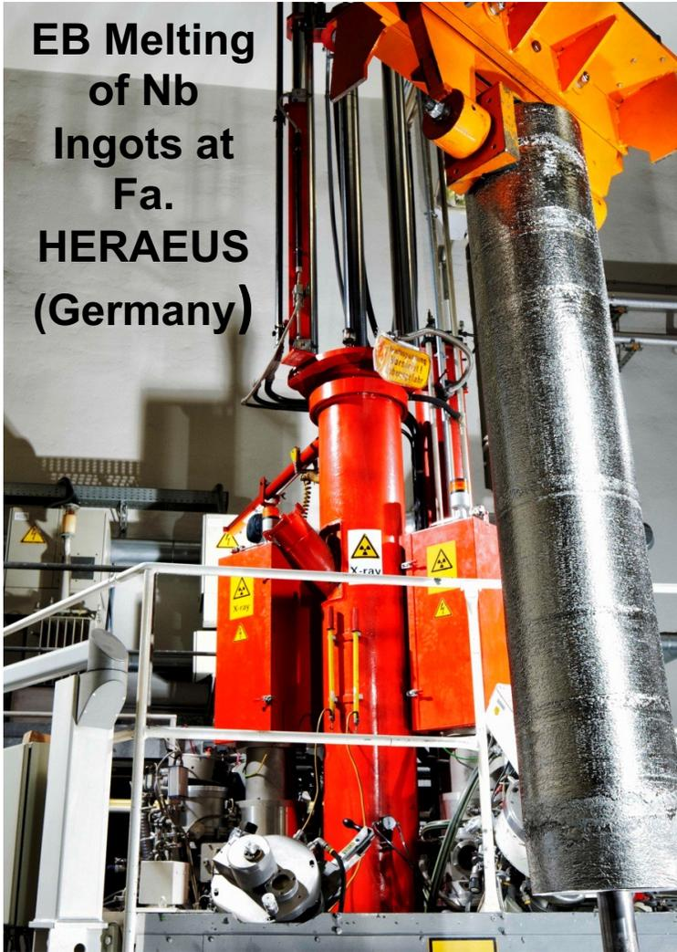
As a result of the increasing demand for refractory metals in the last few decades, the electron-beam furnace has been developed to a reliable, efficient apparatus for melting and purification.
