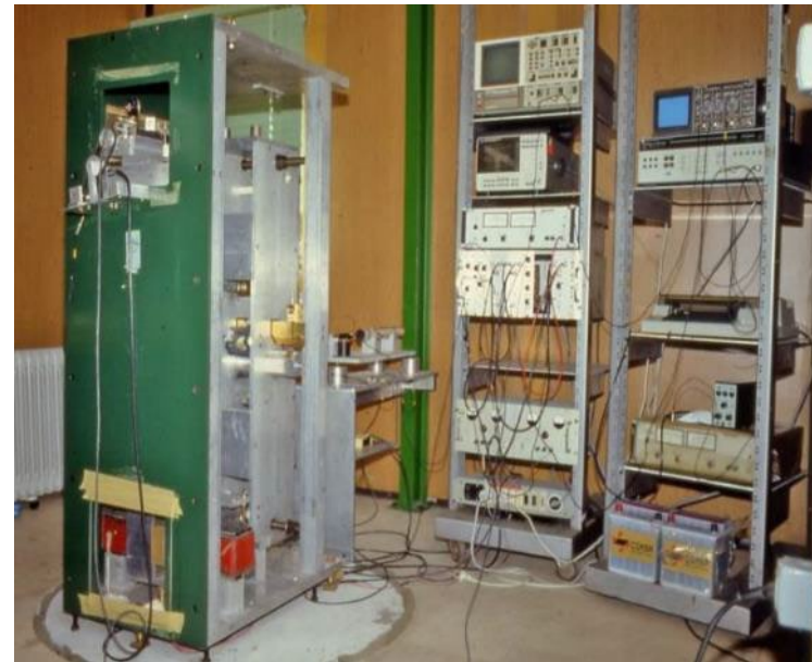
Seismic isolation for resonant bars Going low in frequency to detect pulsars
