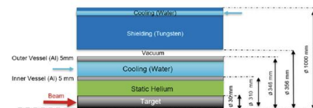
Figure 2 schematically details the bodies, dimensions and materials of the current proposal.
