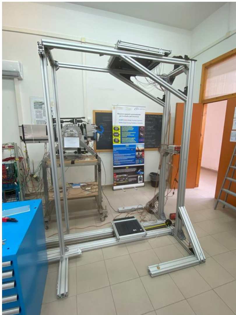
DAQ with TOP-BOTTOM fourfold coincidence
