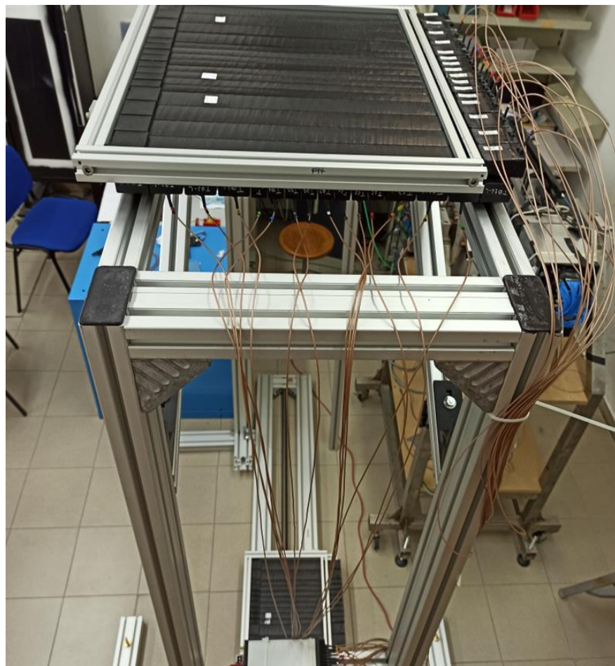
DAQ with TOP-BOTTOM fourfold coincidence
