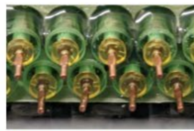
6. Final sealing with stycast Glue.(vertical position)
