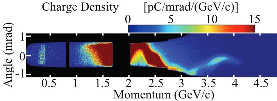
2014: Capillary discharge produced beams up to 4 GeV
