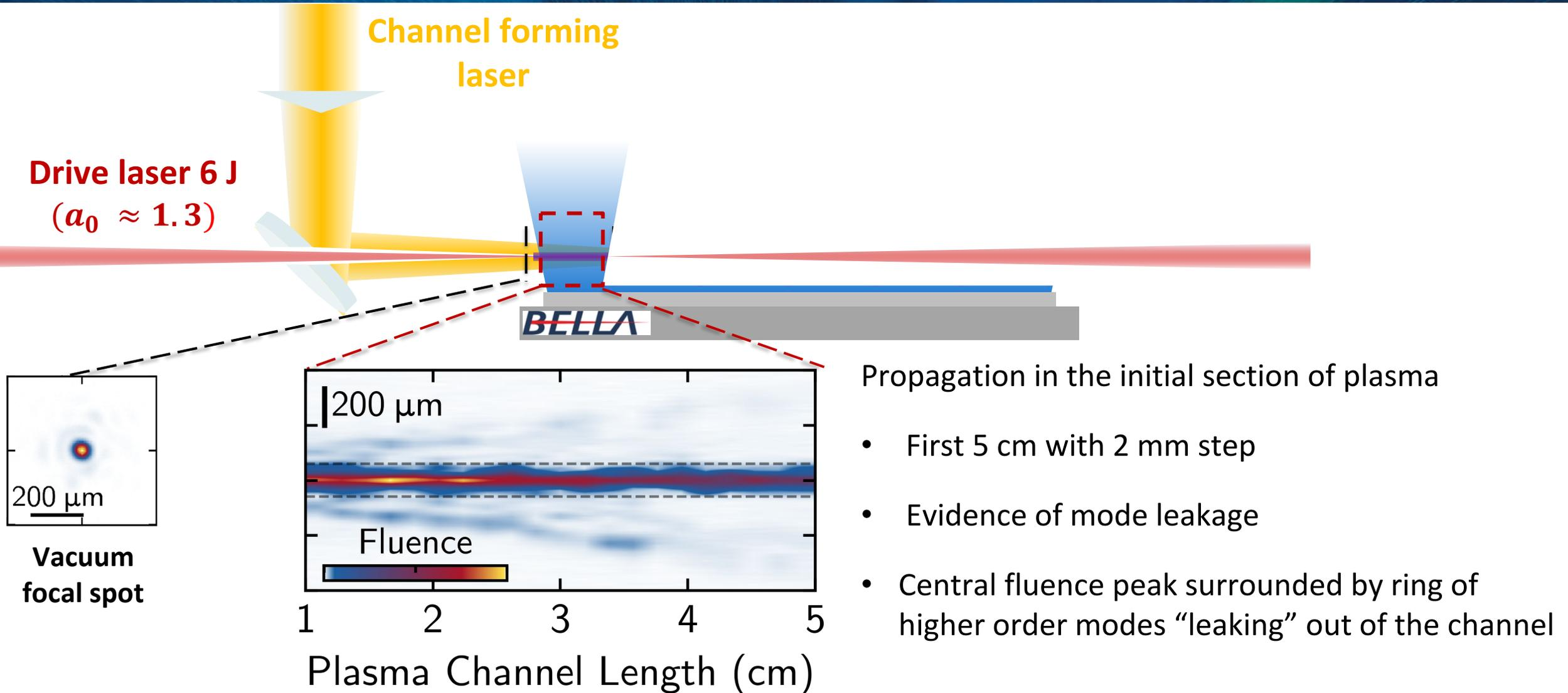
Propagation in the initial section of plasma
