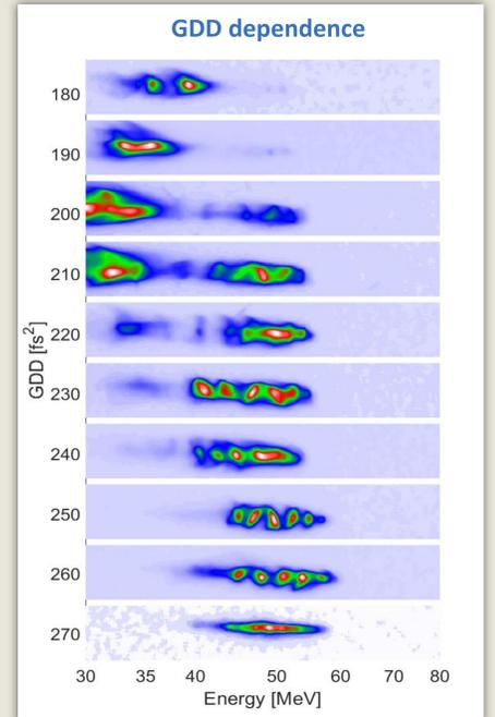
Selected shots from two distinct scans of 10 shots per setting. The counts have been normalized for each shot to better display the behavior of the modulations and their energies. While changing the pressure, the GDD was kept at 250 fs<sup>2</sup>. Below 8 bars, no electrons were detected. For the GDD scan, the pressure was 9 bars.
