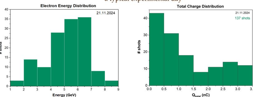
In this example, 137 shots were fired, and different parameters were scanned to find optimal electron acceleration conditions.
