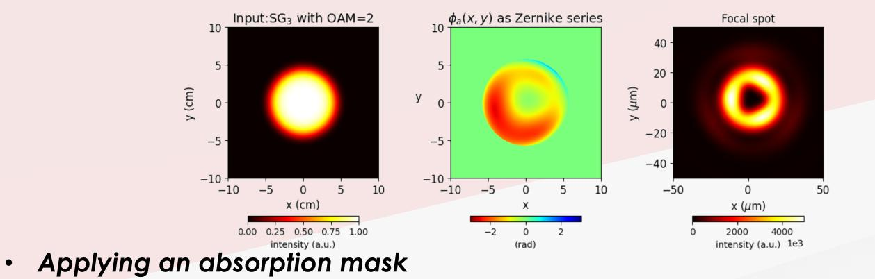
Phase masks are given as 2D matrices; in the plots '1' means absorption.
