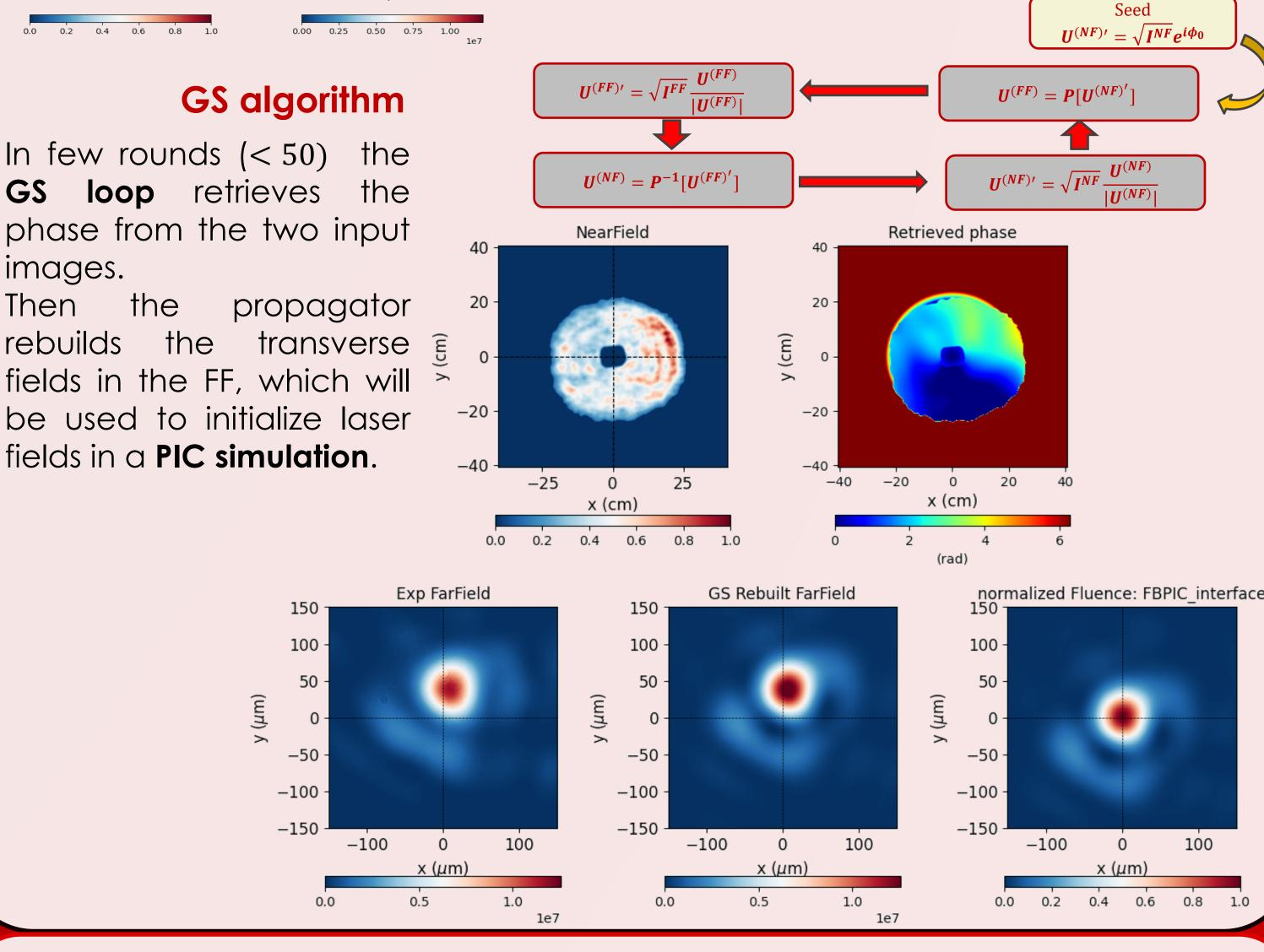
The phase map  $\phi(x,y) = m\theta(x,y) + \phi_a(x,y) + \phi_{mask}(x,y)$  can include an Orbital Angular Momentum (**OAM**) m, an aberration phase  $\phi_a$  given in terms of Zernike series (user provided aberration coefficients) and a user defined phase/absorption mask  $\phi_{mask}$ .
