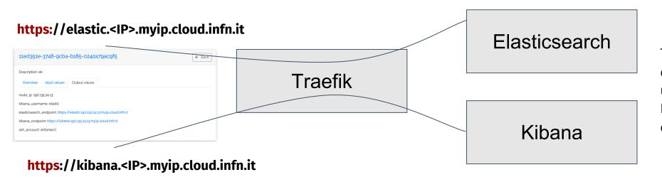
Traefik terminates the SSL connections: it is configured to use an ACME provider (Let's Encrypt) for automatic certificate generation.
