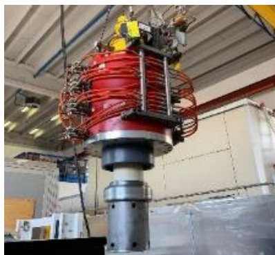
CPI VKX8311A Klystron (50 MW, 50Hz)
