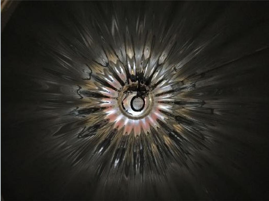
Muons are stopped in a slanted BC400 170  $\mu\text{m}$  thick target with 6 holes and a pattern of dots (photographed by a camera) to continuously monitor the shape and position of the foil
