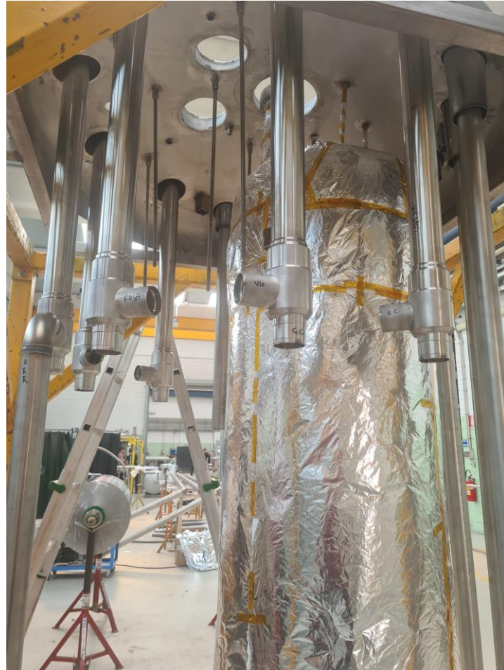
Fig. 1 – Ongoing manufacturing activities: HR valve box, inner vessels wrapped in MLI, internal structure and HEX installed (left); LF valve box, B4110 Cu filter wrapped in MLI, piping disassembled for welding + X-rays (middle); HR, LF, and NP piping sub-assemblies ready for X-rays (right).
