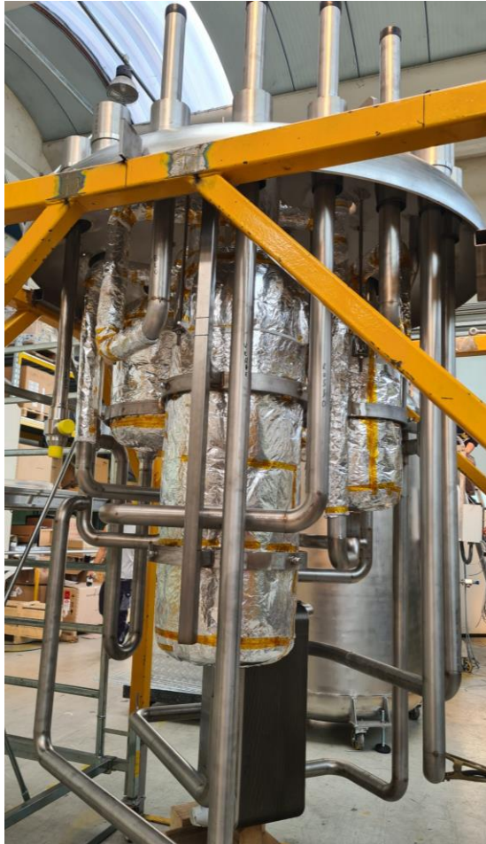
Fig. 1 – Ongoing manufacturing activities: HR valve box, inner vessels wrapped in MLI, internal structure and HEX installed (left); LF valve box, B4110 Cu filter wrapped in MLI, piping disassembled for welding + X-rays (middle); HR, LF, and NP piping sub-assemblies ready for X-rays (right).
