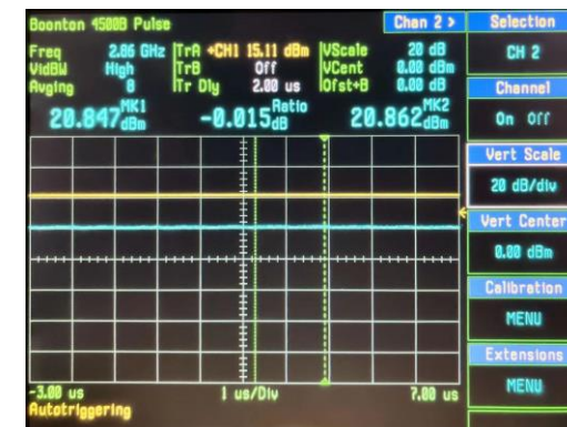
Fig.39 The measured 2.855132 GHz microwave power output from the PSG
