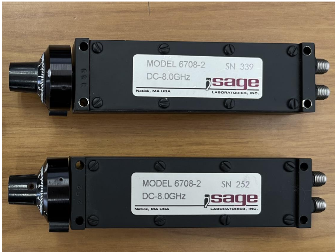
Fig.49 Sage 6708-2 mechanical phase shifter
