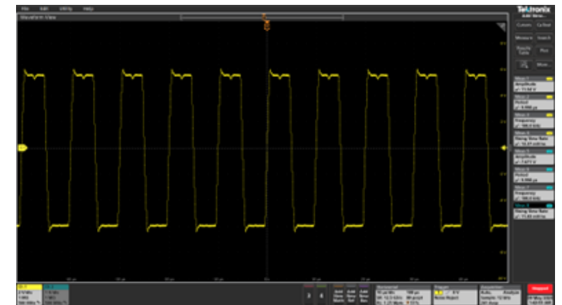
Fig.54 100 kHz error waveform under 2.85132 GHz microwave modulation
