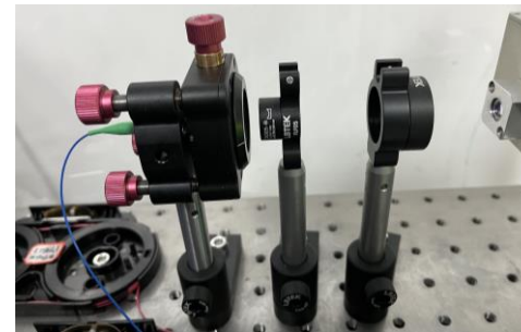
Fig.8 Beam reducer and collimator
