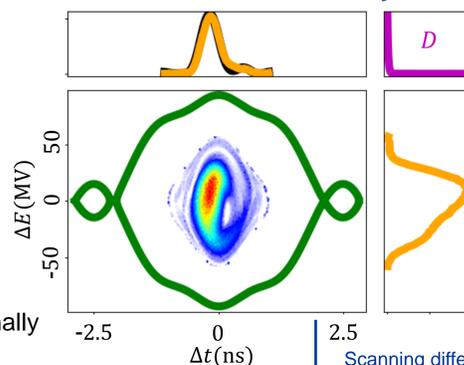
Calibration using a 4-D minimizer algorithm for the discrepancy
