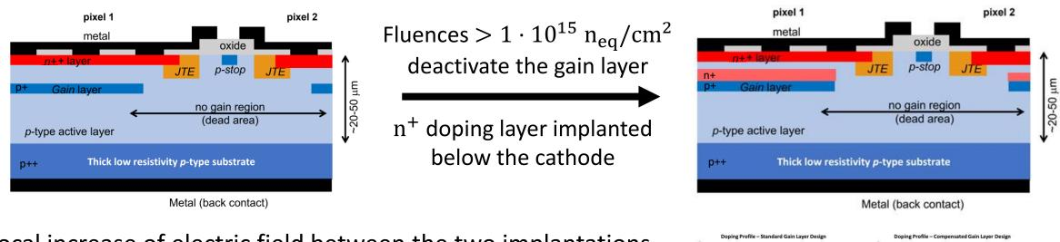
Local increase of electric field between the two implantations allows signal multiplication
