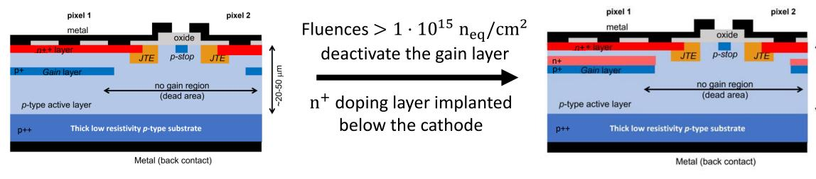
Local increase of electric field between the two implantations allows signal multiplication
