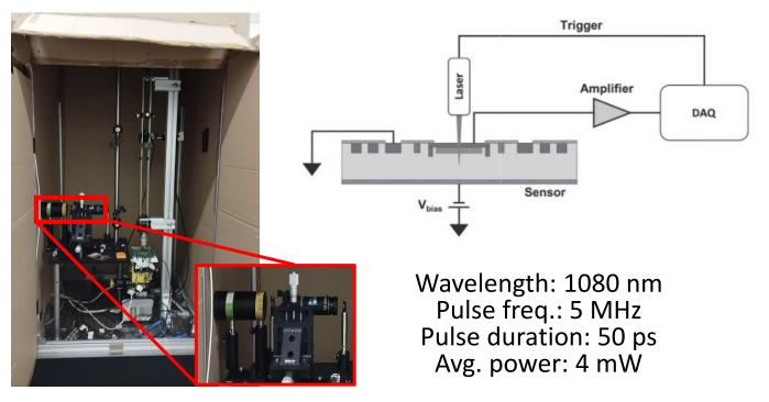
At the moment, I am commissiong the setup through gain measurements on standard LGADs
