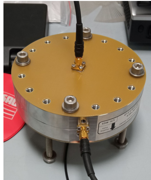
Configuration setup to test the ICT with the pulser
