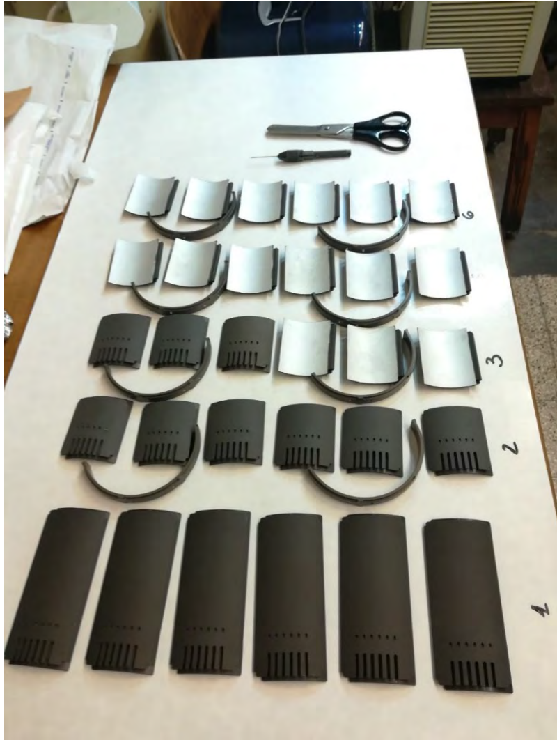
Tiles' internal view (conductive aluminum)
