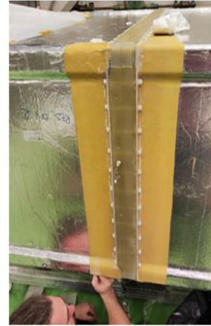
High Voltage feedthrough external connection
