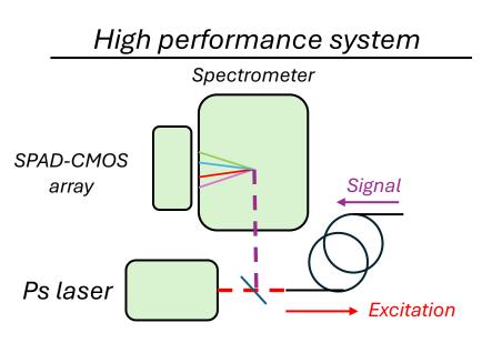
Ps pulsed laser < 100 ps *15 keuro* Spectrometer *10 keuro* SPAD-CMOS 320x1, 17 ps tagging, 2 ns gate *27.5 keuro* Optics and filters *3 keuro*
