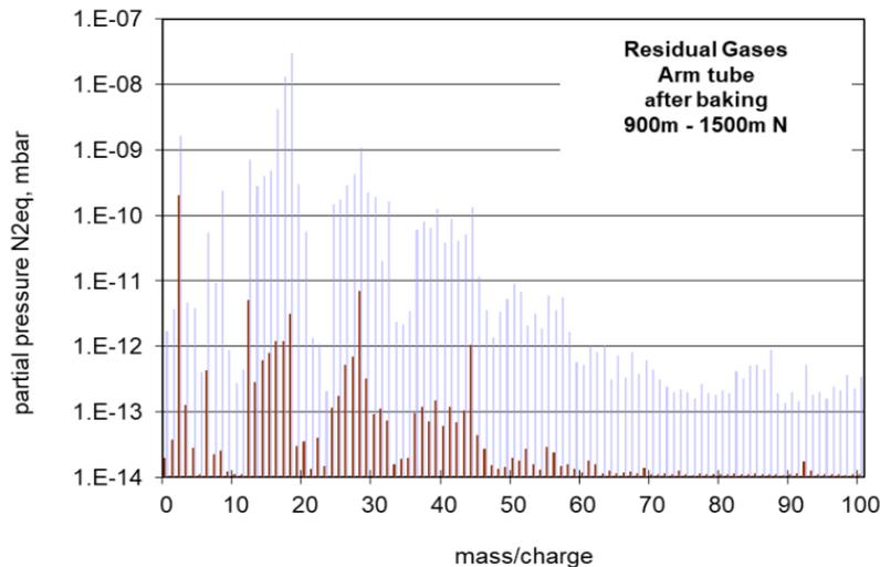
Accumulated gas over 2+ years on a 'tube prototype'
