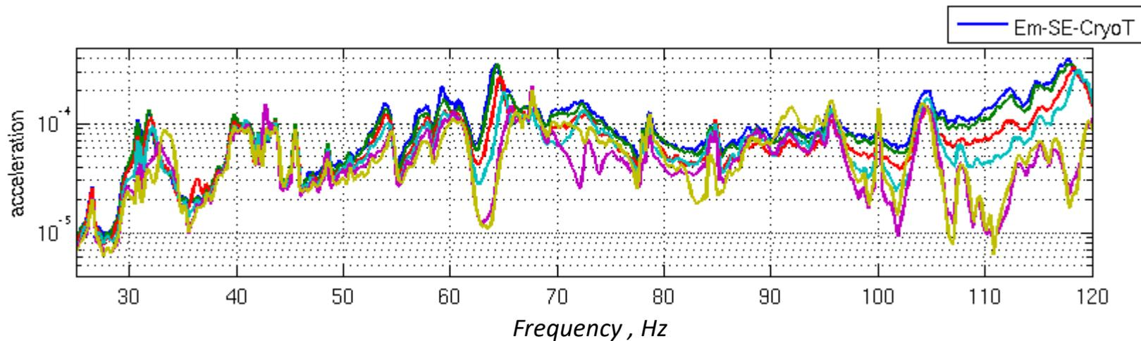
*Increase of the seismic vibrations of cryostat walls due to LN2 bubbling*
