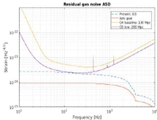
Fig. 1 Estimate of the noise due to the residual gas in the 3 km arms for the present configuration (O3). The Adv goal is added for comparison. The partial pressures in the computation are reported in tab.1.
