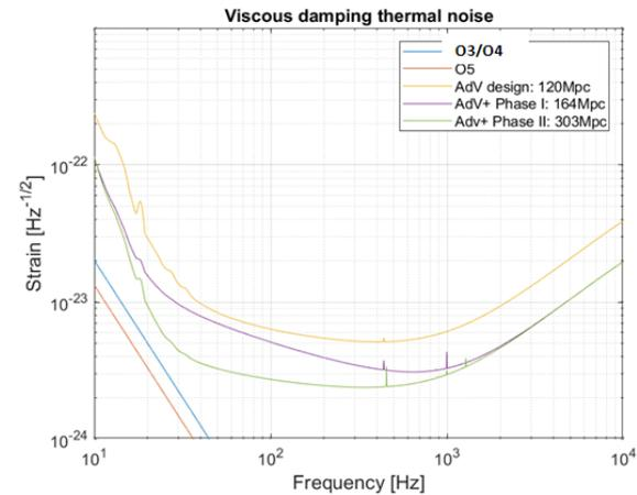
Fig.1 Strain equivalent noise amplitudes for the two considered scenarios, compared with some sensitivity predictions. The parameters used in the computation are reported in tab.1.
