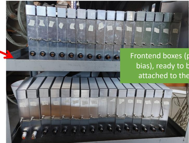
Frontend boxes (preamp and bias), ready to be directly attached to the cryostat
