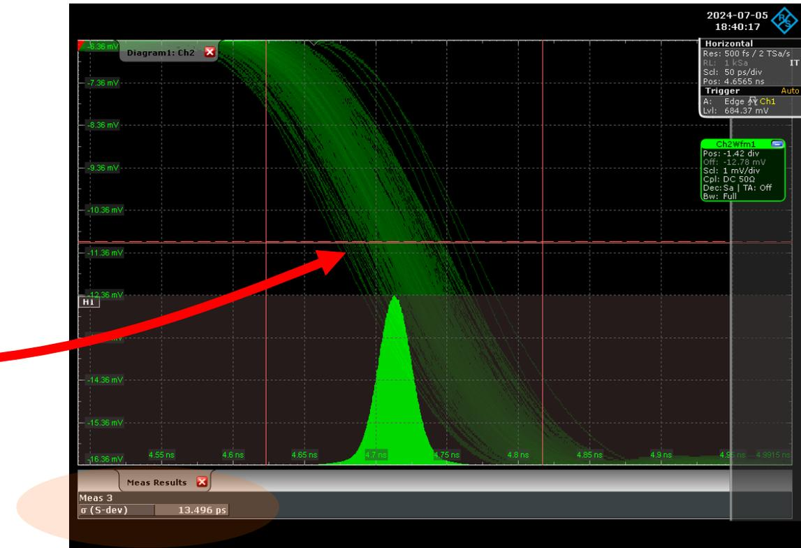
Jitter reale a 300 K, considerando 10.3 ps<sub>RMS</sub> strumentali: 8.7 ps<sub>RMS</sub> (a 77 K ~ 21 ps<sub>RMS</sub>)
