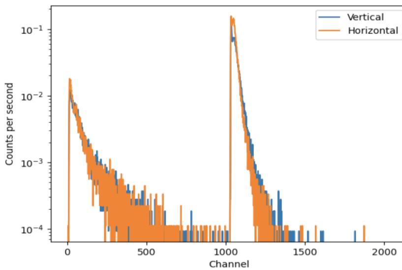
Example of the PSD output. The channels in the range 0-1000 represent the pulse high spectrum for the neutron signal. The channels in the range 1001-2000 represent the pulse high spectrum for the muon signal. The neutron signal is independent of the detector position. The muon signal is, as expected, lower for the vertical position.
