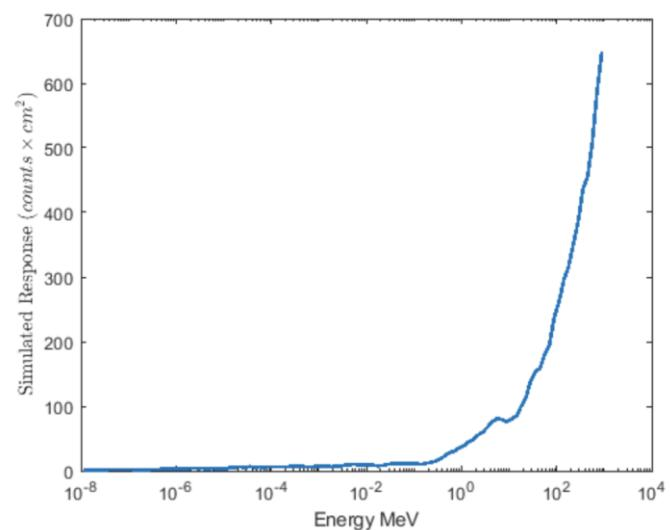
Simulated response function in counts per unit of neutron fluence
