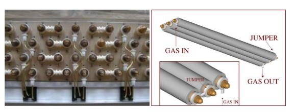
To ensure stable and uniform drift properties, the leak rate at room temperature should not exceed 2x10<sup>-8</sup> bar l/s per tube
