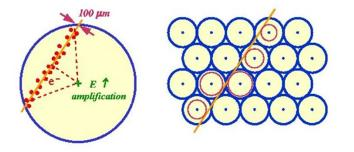
Original MDTs = diameter 3 cm (1076 chambers), Small MDT (sMDT) = diameter 1.5cm (22 chambers)
