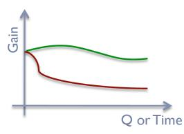
Ageing depends on the total collected charge Q:  $Q[C] = Gain \times Rate \times Time \times Primaries$ Rate of Aging: R(%) ~ slope of Gain vs. Q where Q is expressed in [C/cm] for wire detectors and [C/cm<sup>2</sup>] for strips or continuous electrodes.
