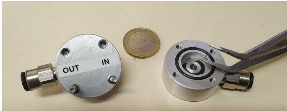
The valve is made of aluminum the screw are in stain steel, the gas connections are in brass the O-ring in NBR the same used in all the gas connectors of the present distribution.
