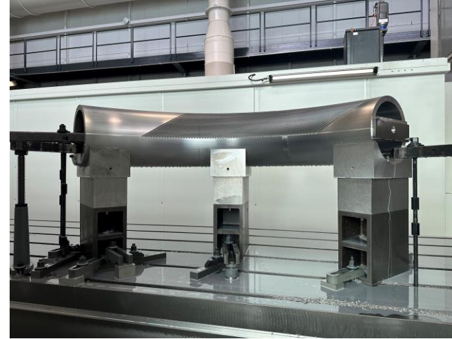
Machining of 3-part inner mandrel is completed
