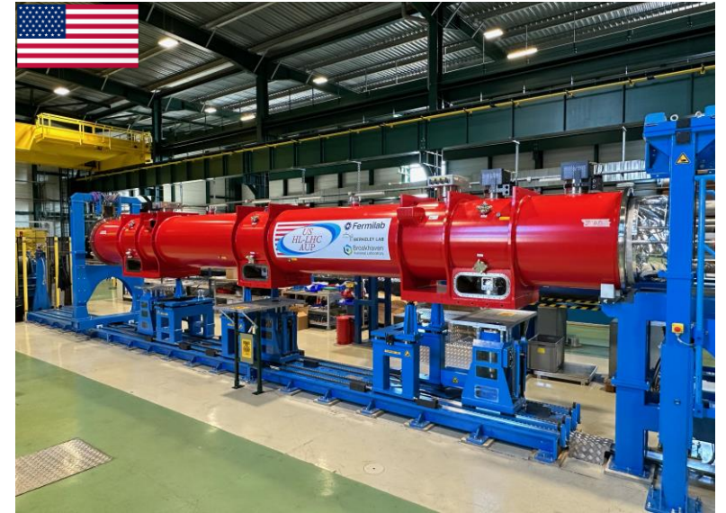
First AUP LQXFA01 cryomagnet mounted on Cryostat Tooling in SMI2 at CERN
