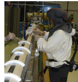
Ceramic binder application by brushing
