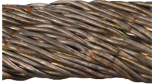
Short-twist-pitch cabling pattern for ITER CS Courtesy of C. Sanabria (formerly FSU)
