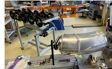
Winding of sub-scale Fusillo model
