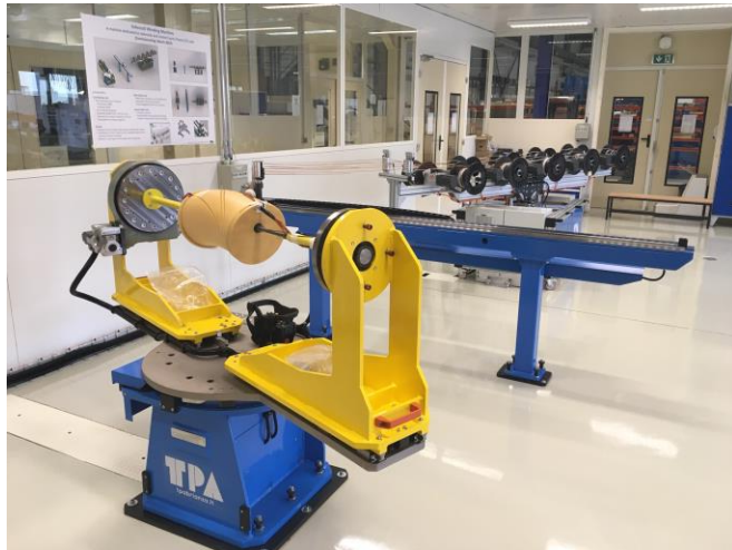
Commissioning of new winding machine is underway at CERN
